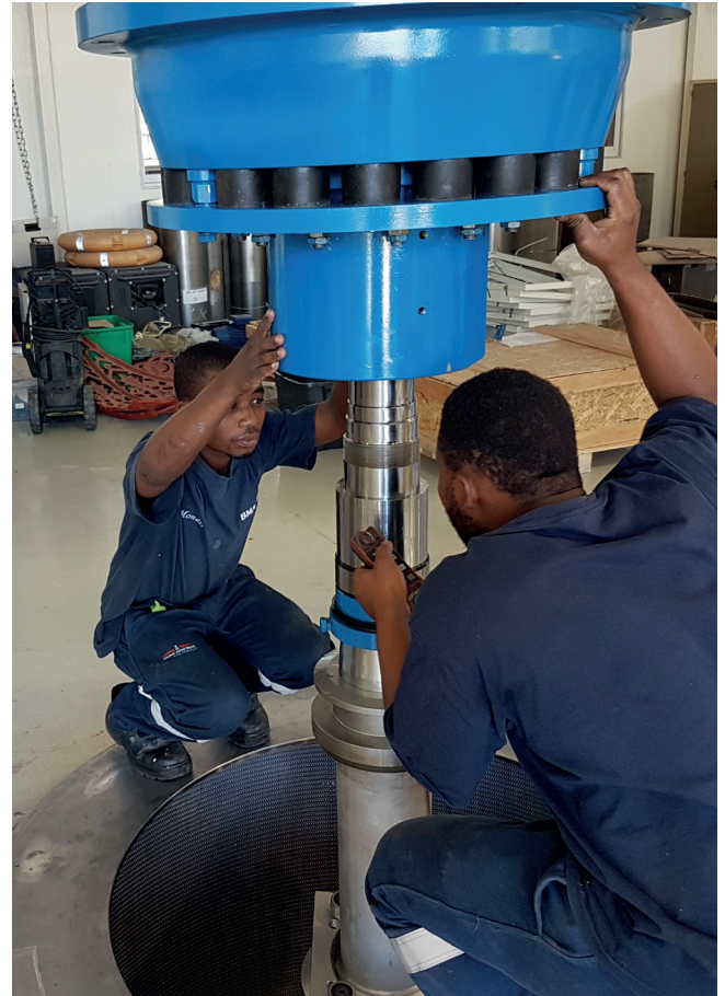
Workshop maintenance on an E1810 centrifugal
