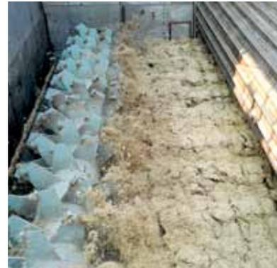
The diffuser from BMA is a fully enclosed, stand-alone horizontal chain conveyor with a rectangular cross section. Its top cover is designed as a rounded steam dome; a special base facilitates the juice flow.
