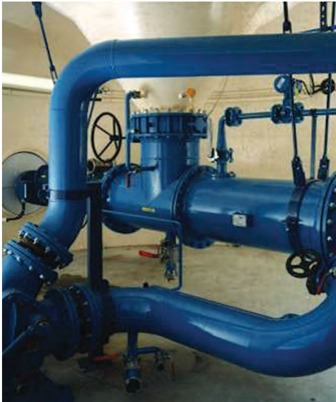
Figure 3. BMA molasses-magma mingler (MMM)
