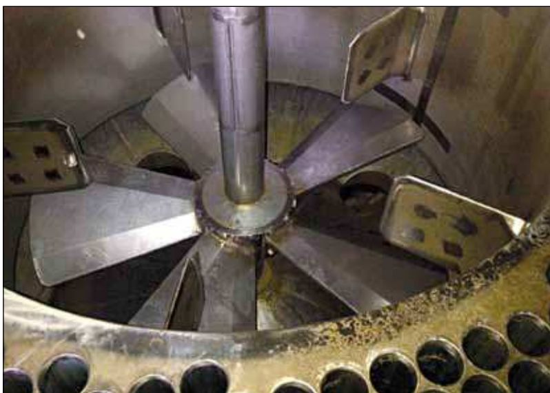
Figure 3. The five bladed impeller found in chambers 3 and 4
