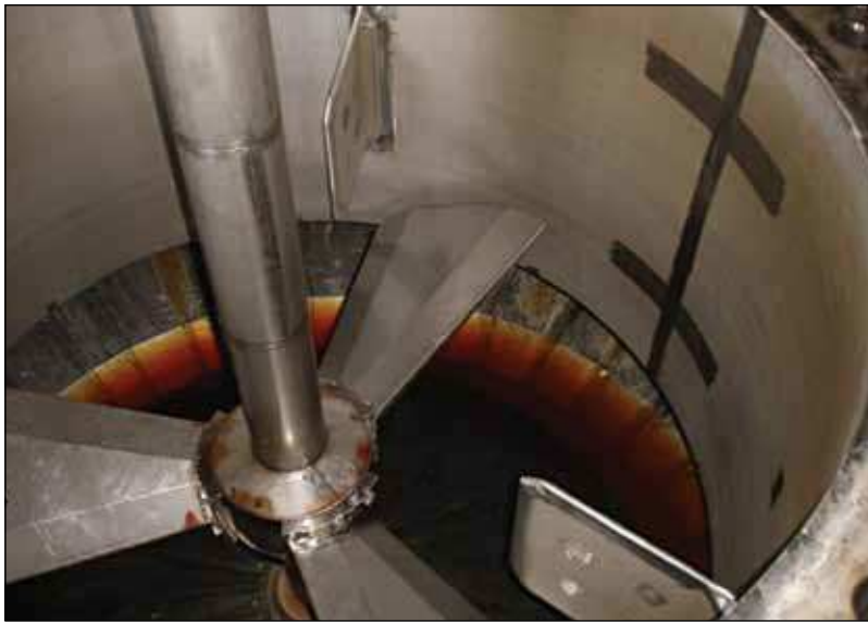
Figure 2. The three bladed impeller found in chambers 1 and 2
